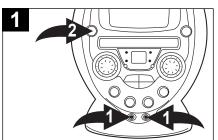
Insert the microphone into Microphone 1 or 2 jack • and press the POWER button • on the main unit...
